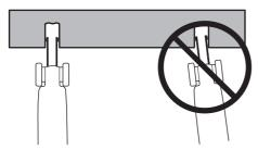
Always cut from top to bottom (A). Remove the cutter and use a crowbar to remove the material that remains between the cut (B).
